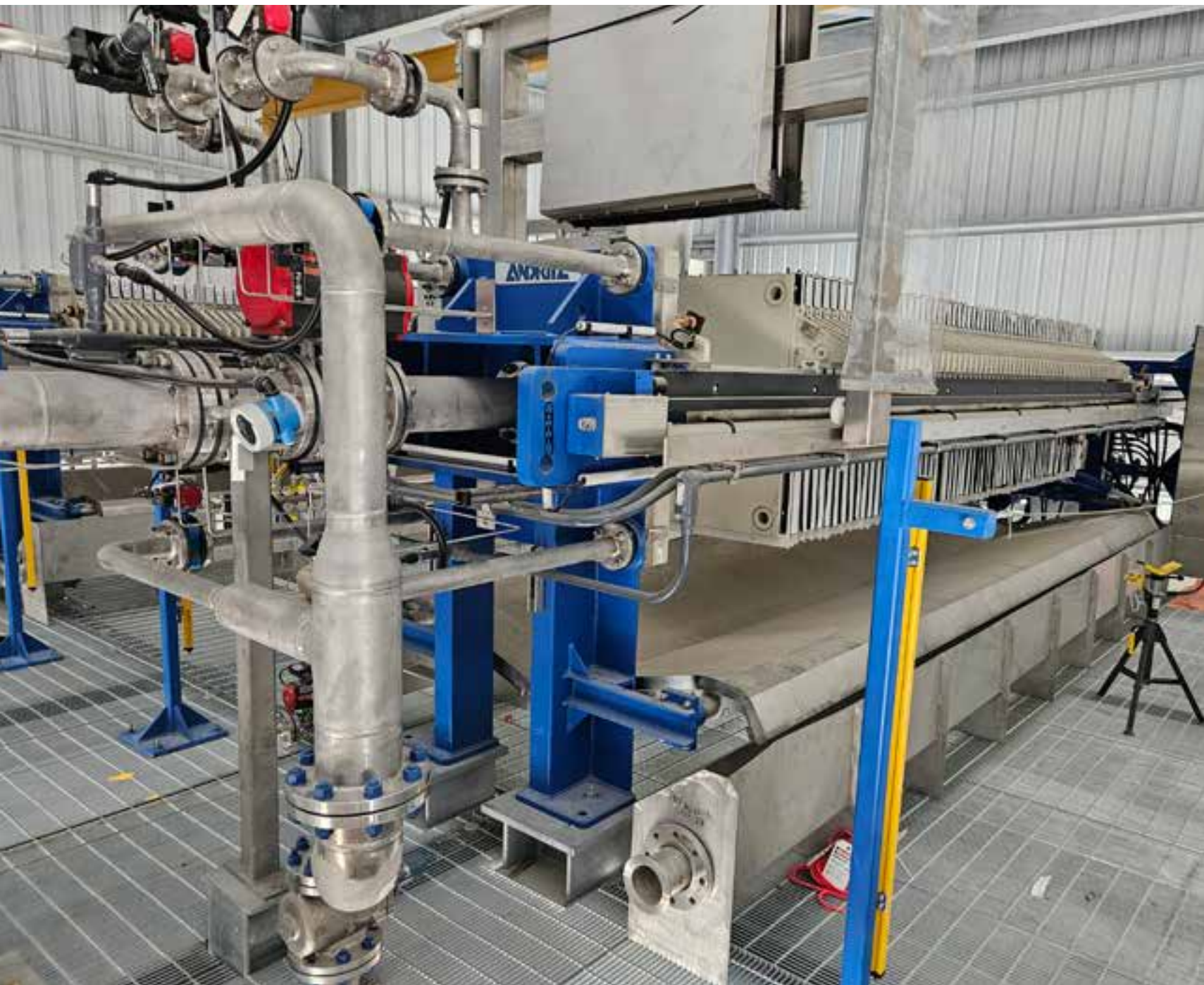
Veolia’s versatile sludge dewatering facility contains ANDRITZ filter presses and screw presses, designed to efficiently process varying sludge compositions.
