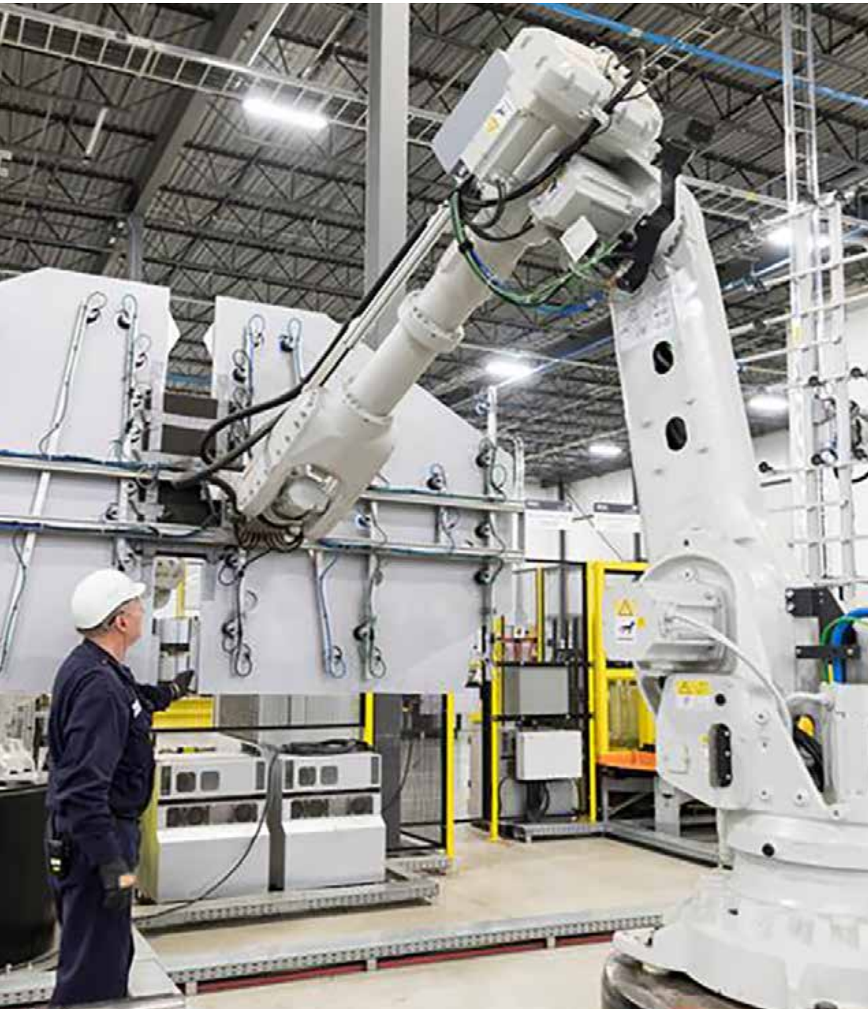
ANDRITZ's SOURING laser welding system at ArcelorMittal produces lightweight automotive door rings, achieving 30% weight reduction through innovative tailor-welded blank technology.
